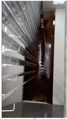
Horizontal spray of aluminum profile
